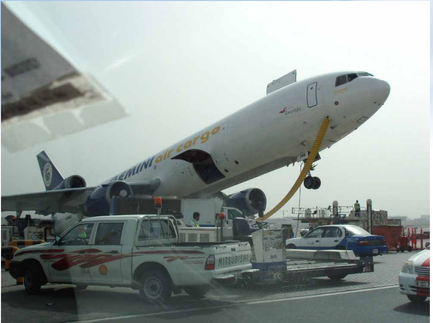
A Gemini air cargo flight was being loaded when a number of containers got shifted towards the tail of the aircraft upsetting the balance of the aircraft and its nose went into the air.
