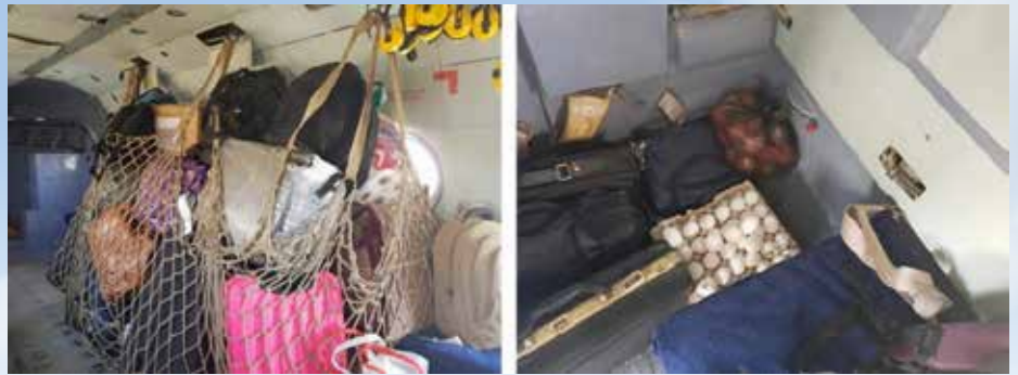
Overloaded and unsecured items inside the helicopter
